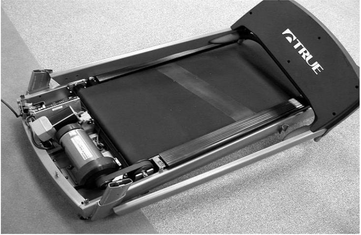
Detach the rubber band from the upper wiring harness and route the cable down the pedestal leg support and out the bottom hole as shown.
